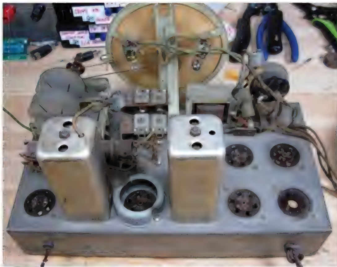
Bare radio chassis with tubes removed.
